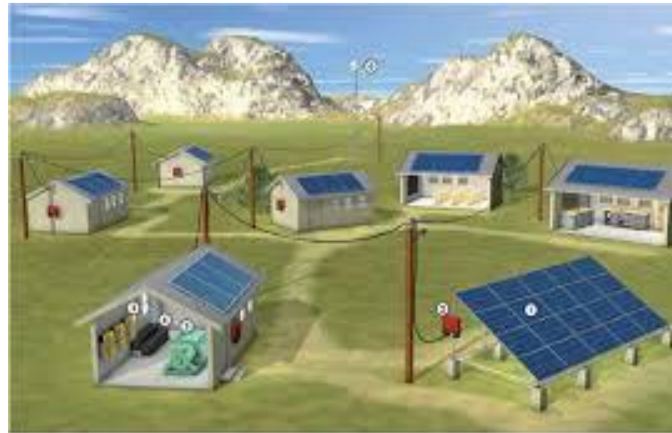
Components: 1. PV array, 2. SUPPLY BUS, 3. SUPPLY CABLE, 4. Recharge, 5. Diesel generator, 6. Wind turbine system
